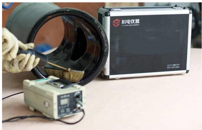
High Voltage test to check integrity of glass lined equipment
