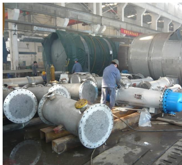
Monitoring manufacturing process of hastelloy heat exchangers(a cost engineered design made by Raschka Engineering)
