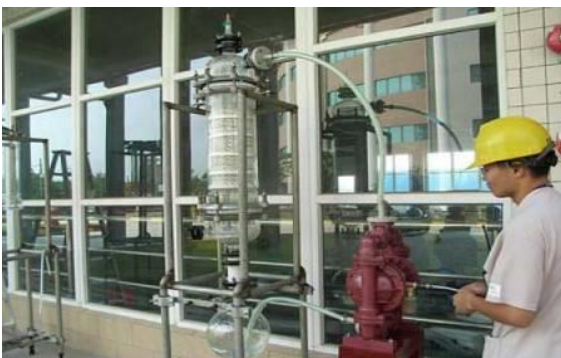
Testing of ceramic column packing (8 out of 10 samples failed the pH range tested!)
