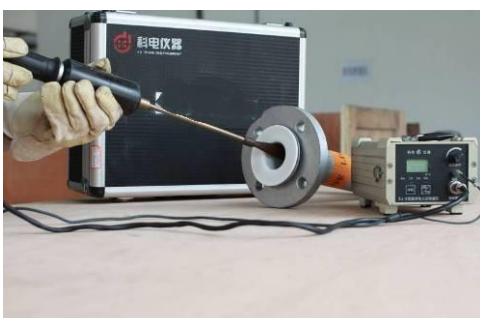
Material test on PTFE lined pipes and fittings
