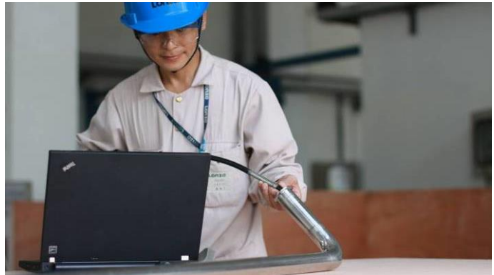
Check and document welding quality inside tube (Boroscope)
